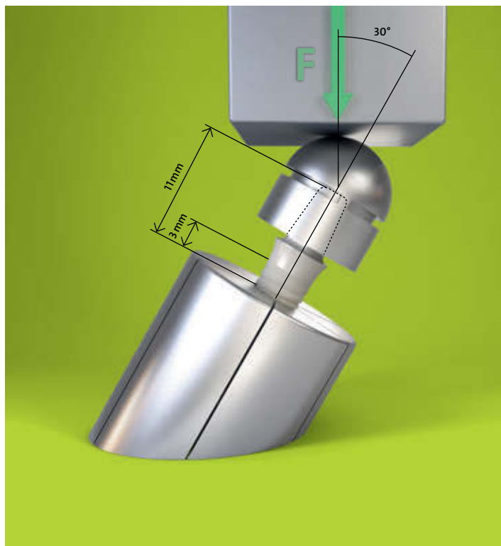
Fig. 1: Test setup according to ISO 14 801
