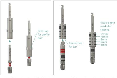
Only Profile Drills and Taps labeled to be "FIBA compatible" are to be used with the Guided Adapter, FIBA. Always use the correct Guided Adapter according to the T-sleeve position (H2, H4, H6). Using the incorrect Guided Adapter or a non-FIBA compatible component may result in an incorrect drilling depth.
