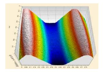
FIGURE 10. Confocal laser scanning microscopy in the screw thread region.  $^{14}$
