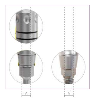
Step 3 - Final positioning of the implant
