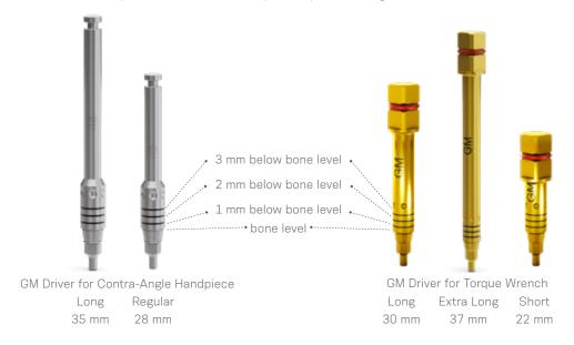
**Note 1:** There are 3 similar markings at 1 mm intervals in the Drivers for the Contra-angle handpiece and Torque Wrench. These markings guide the depth of the final positioning of the implant in the following way: first stripe for 1 mm below bone level, second for 2 mm and third for 3 mm. Each full turn of the implant results in: (a) 2.2 mm for the Drive implants; (b) 1.4 mm on average for the Helix™ implants; and (c) 1.2 mm for the Titamax implants.
