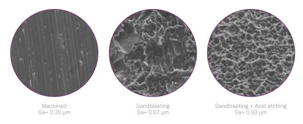
FIGURE 8. Physical manufacturing process for the Neodent® surface treatment.
