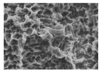
FIGURE 9. Micro (0.3 - 1.3  $\mu$ m) and macro (15 - 30  $\mu$ m) roughness for Acqua and NeoPoros.
