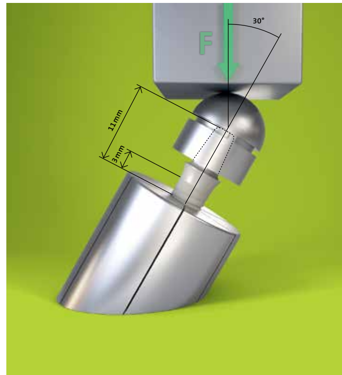
Fig. 1: Test setup according to ISO 14801
