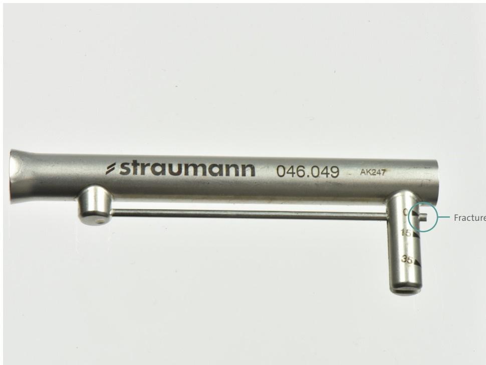
Fracture of a Torque Control Device
