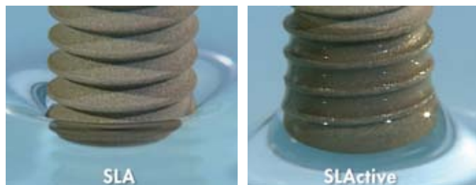
Fig. 3: Immersion of Straumann SLA and Straumann SLActive implants in water demonstrates the wetting of SLActive and its meniscus at the water-air implant interface.
