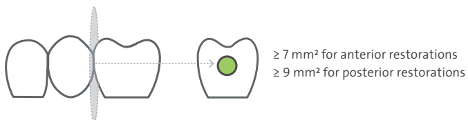
Connector cross-section
