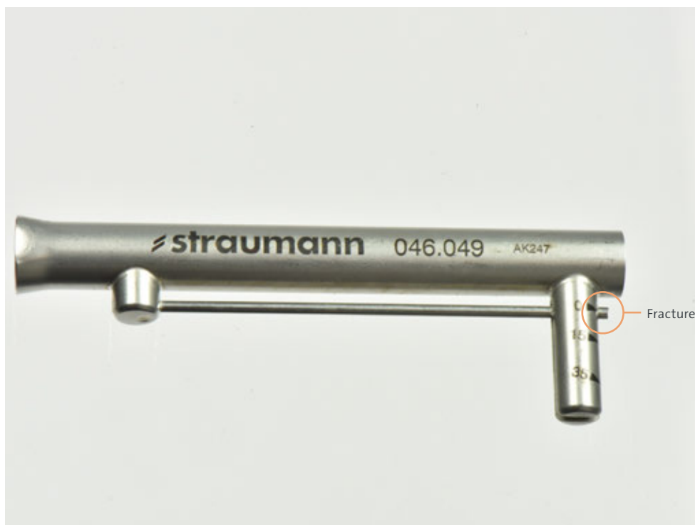
Fracture of a torque control device
