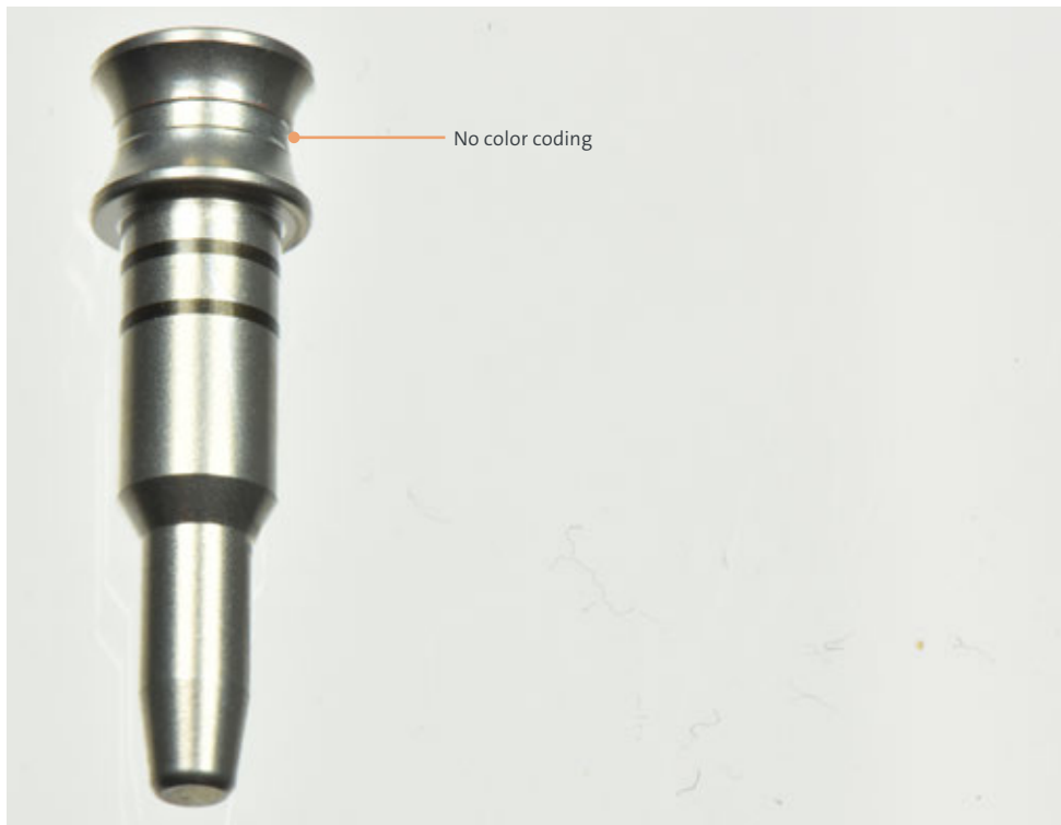
Discoloration of a template fixation pin
