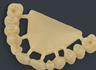
Example of a full arch bridge with a sintering core
