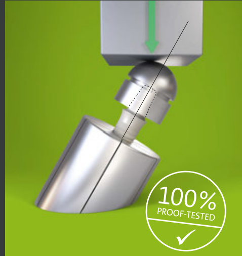
Fig. 1: FATIGUE STRENGTH is the long-term capability of the implant to withstand normal masticatory forces. Next to excellent static strength, the Straumann® PURE Ceramic Implant exceeds the requirements of an extreme fatigue strength test that corresponds to over 20 years of implant use. (Data on file)
