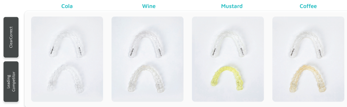
Aligners immersed in their respective substances for 24 hours at 37° C.
