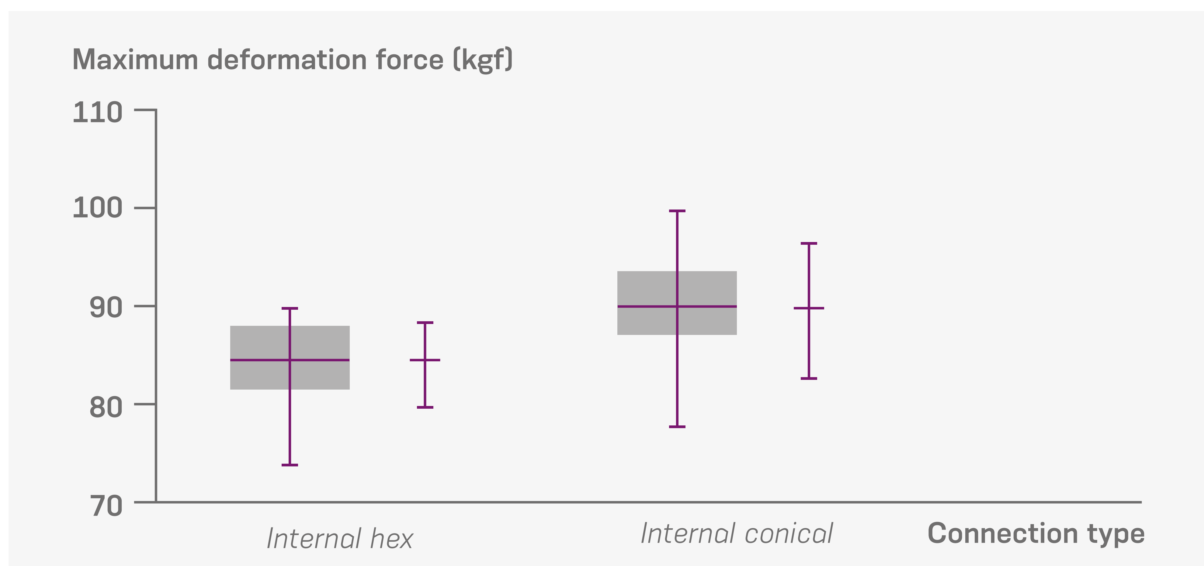
Figure 1: Maximum deformation force values for the internal hex and internal conical systems
