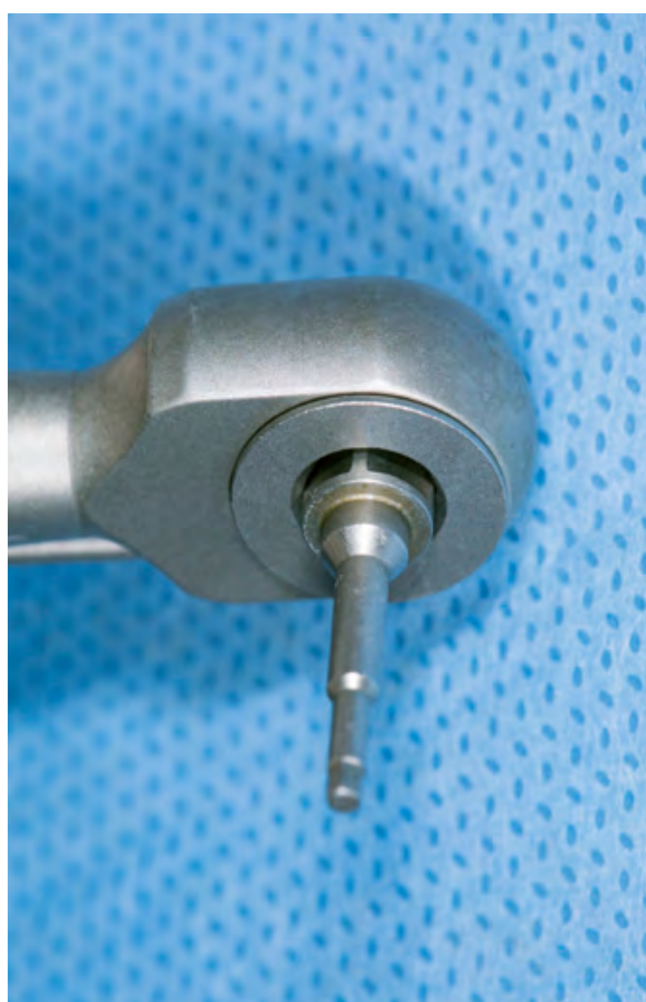
5.c.4 Hex screwdriver torque connection 1.2 mounting to ratchet
