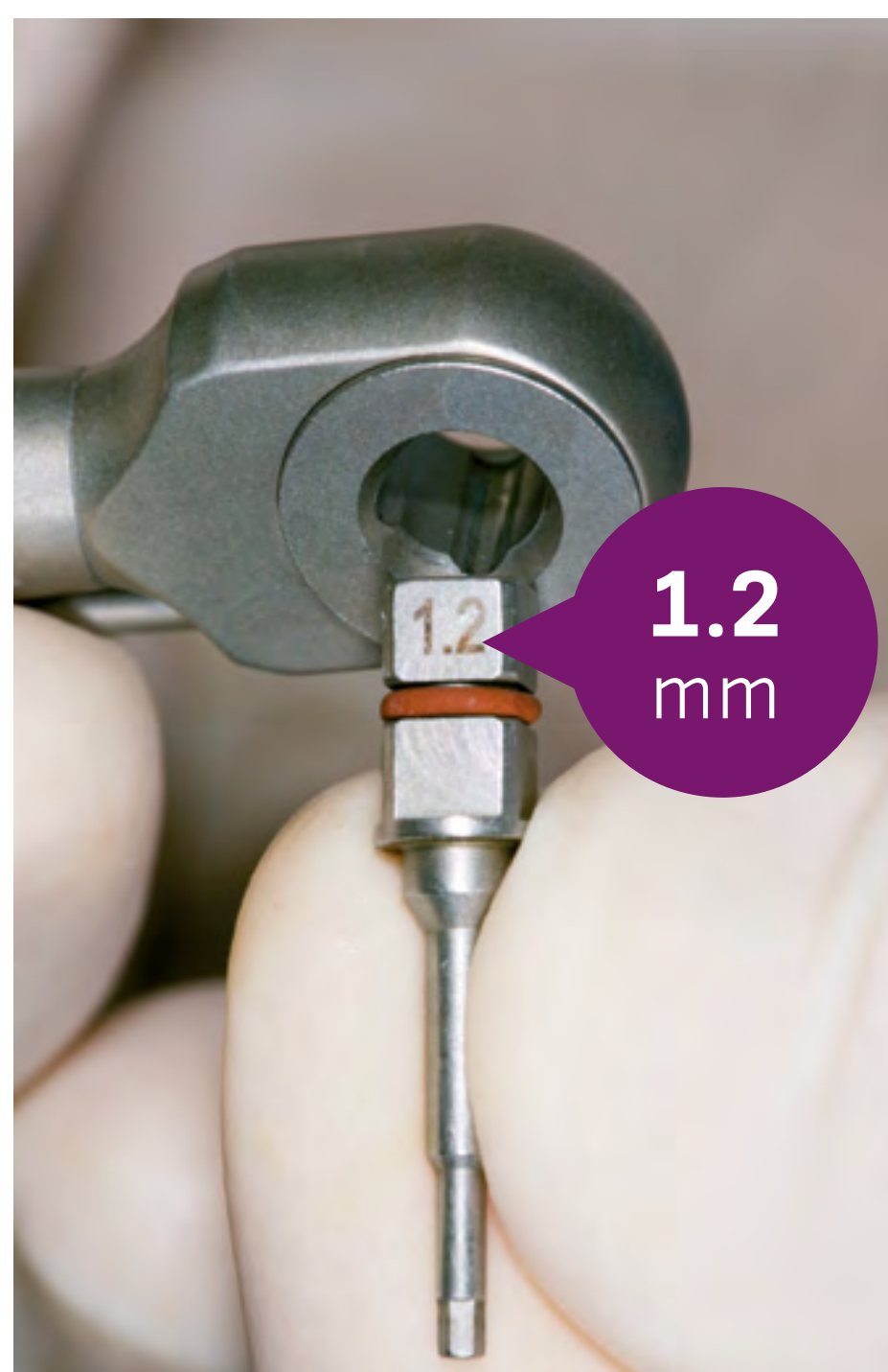
5.c.4 Hex screwdriver torque connection 1.2 mounting to ratchet
